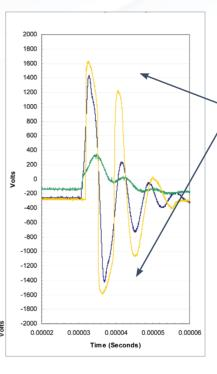
Figure 2: A B3 ring wave at 180 degrees. Notice the yellow and blue lines go above 1200V on both the positive and negative half cycle. This dangerous energy goes directly to expensive electrical equipment.
